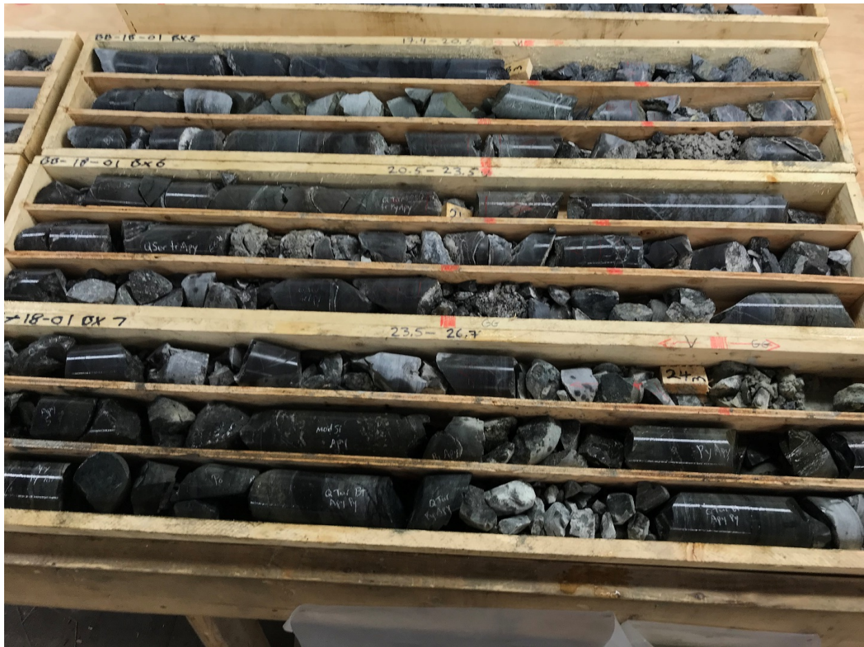
Picture 3—drill cores from 17.4 metres to 26.7 metres at drill hole BB18-01 at Jaxon's Red Springs project, exhibiting very strong silicified and sulphide mineralization.
