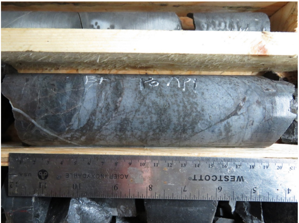
Picture 2—a segment of strong sulphided (Pyrrhotite and Arsenopyrite) tourmalization breccia mineralization core at 21.20 metres from drill hole BB18-01 at Jaxon's Red Springs project.
