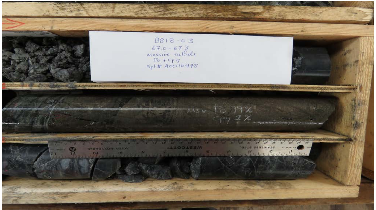
Figure 1 – Segments from 67.0 to 67.3 metres of drill cores from BB18-03 at Jaxon's Red Springs project, which shows very strong silicified and sulphide mineralization.
