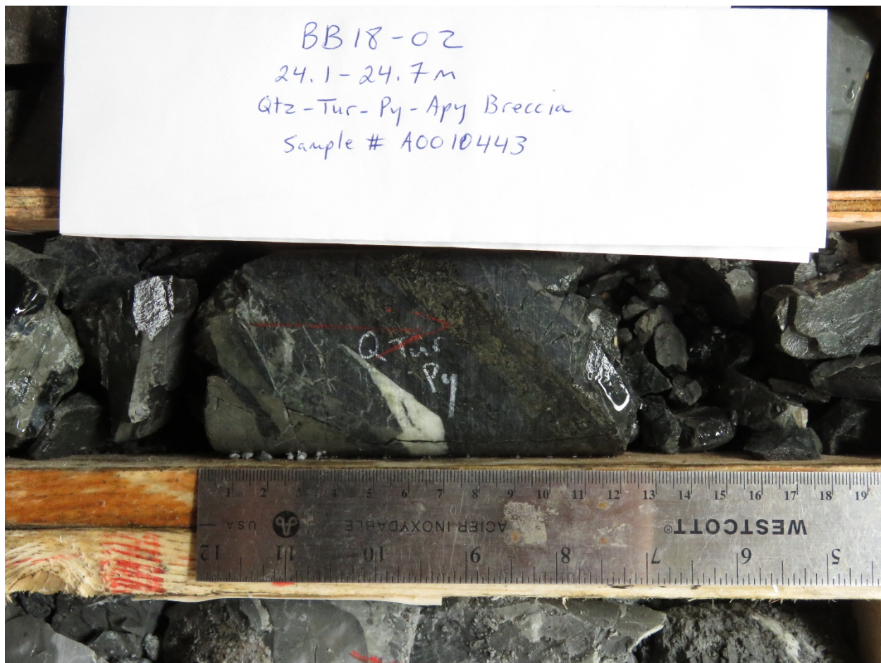
Figure 3 – Segments from 24.1 to 24.7 meters of drill cores from BB18-02 at Jaxon's Red Springs, which shows very strong silicified and sulphide mineralization.
