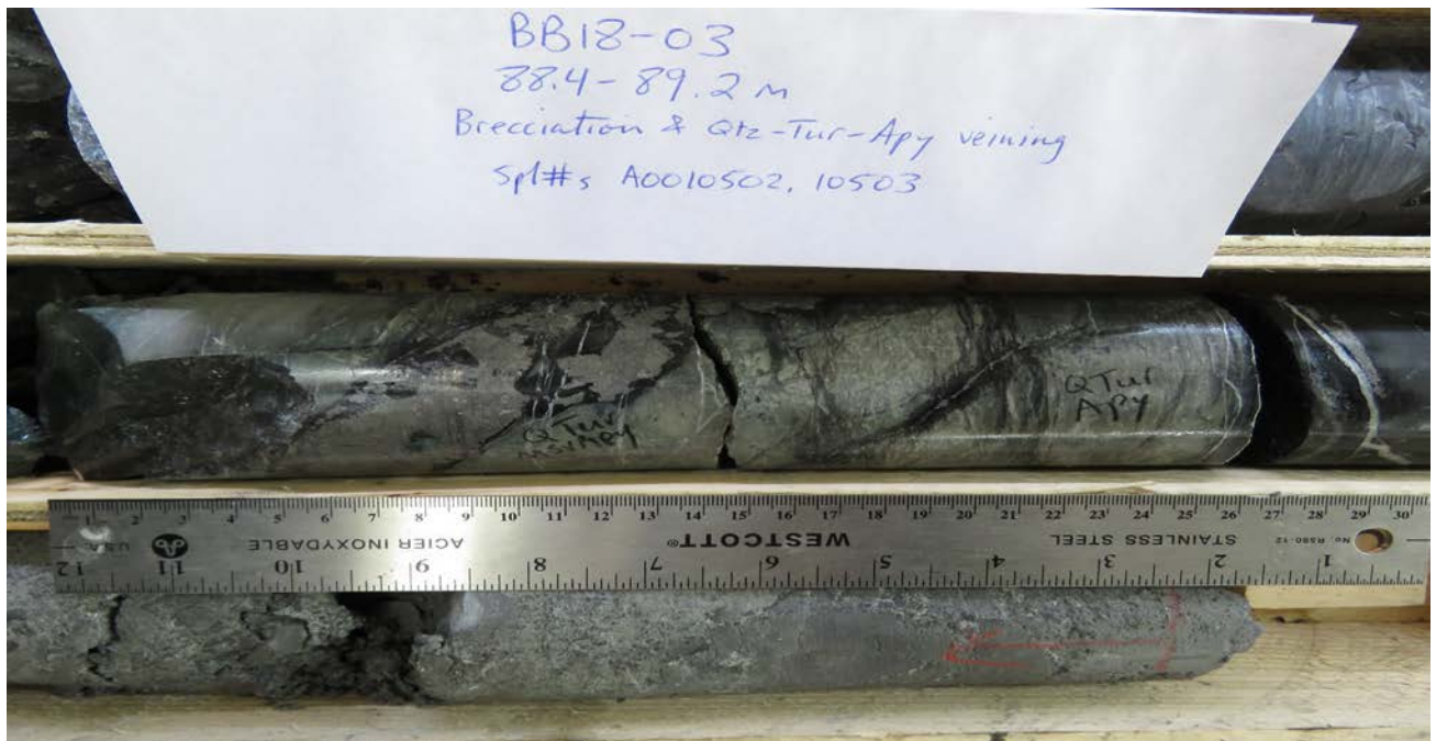
Figure 2 – Segments from 88.4 to 89.2 metres of drill cores from BB18-03 at Jaxon's Red Springs, which shows very strong silicified and sulphide mineralization.
