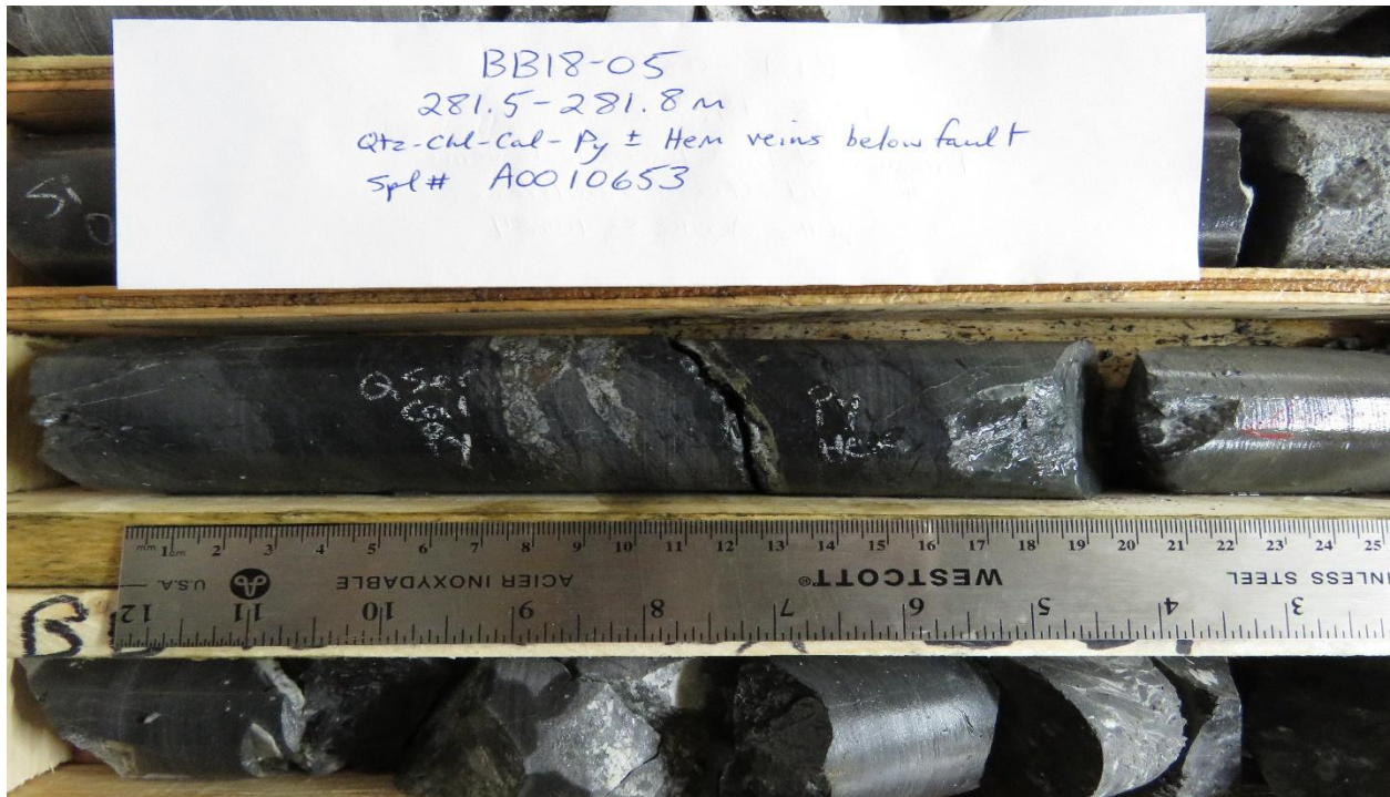
Figure 4 – Segments from 281.5 to 281.8 metres in zone 4 (280.85-294.5 metres of tourmaline breccia) from drill hole BB18-05 at Jaxon's Red Springs Project, which shows silicified and sulphide quartz tourmaline mineralization.
