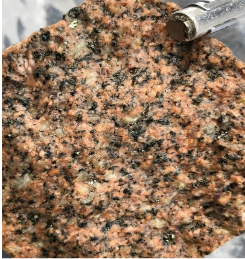
Figure 10: Demagnetised K-feldspar Granodiorite Porphyry Dyke (Outcrop C) with Disseminated Chalcopyrite from the Primary Ridge Target
