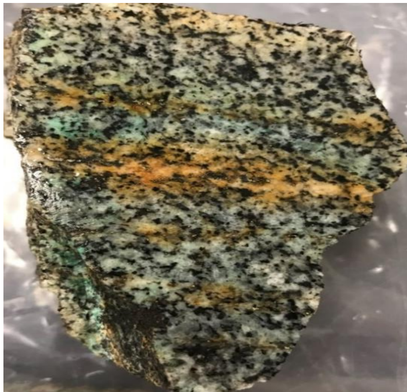
Figure 15: Sample 719511 from the Razorback Porphyry Area. Tonalite with chalcopyrite and malachite alterations, showing a veinlet crossing cut biotite and magnetite veins.
