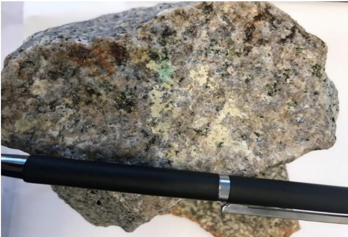
Figure 9: Magnetic Granodiorite with Chalcopyrite and Malachite from the Primary Ridge Target
