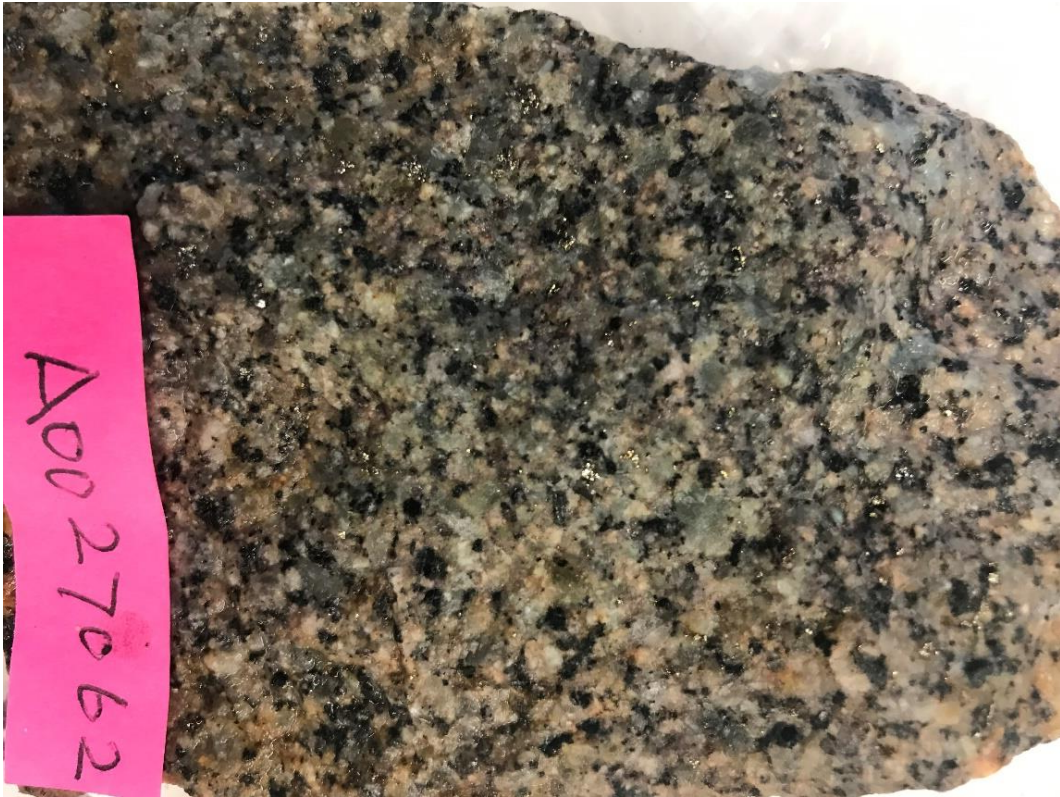
Figure 12: Demagnetized Altered K-feldspar Granodiorite Porphyry Outcrop A from the Primary Ridge Target
