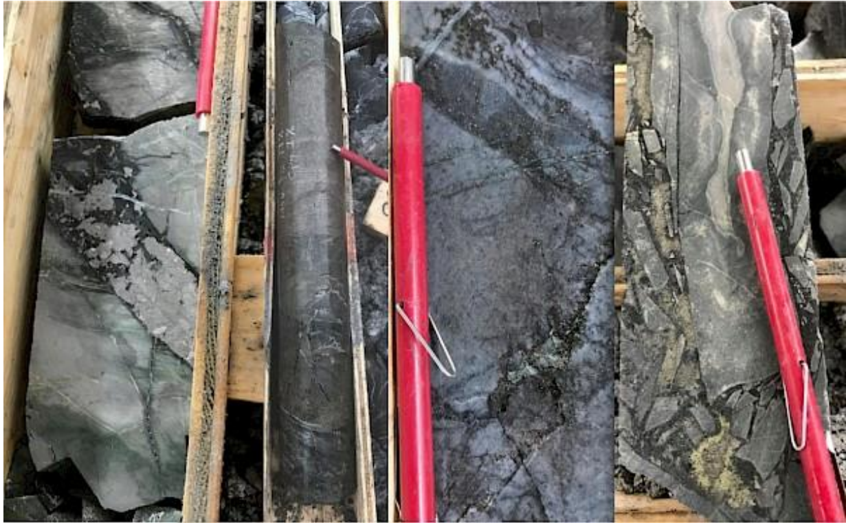
Figure 29: Sulfide Minerals (Arsenopyrite, Pyrrhotite, Pyrite and Chalcopyrite from Left to Right) in Backbone Tourmaline Breccia Drill Core
