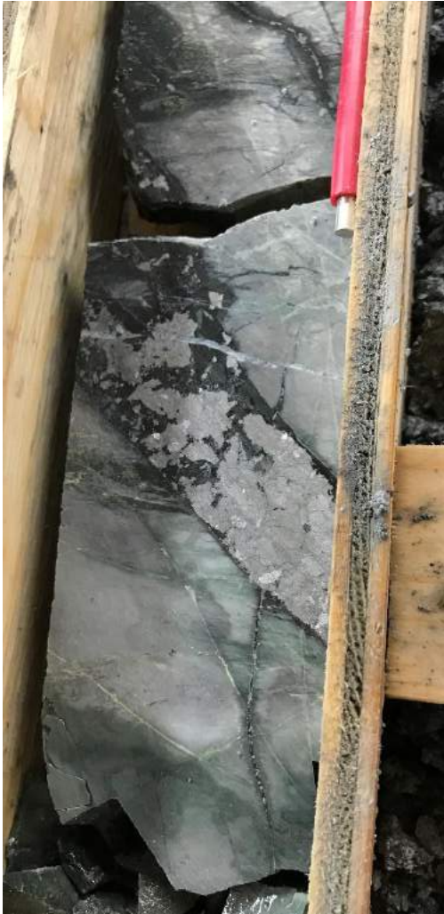
Tourmaline breccia with arsenopyrite at grade of 6.60 g/t Au and 0.10% Co
