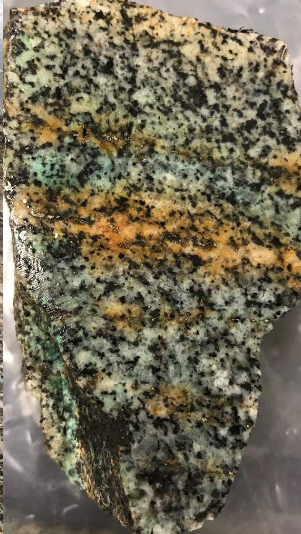
Chalcopyrite, potassium alteration veins & malachite alteration in biotite diorite
