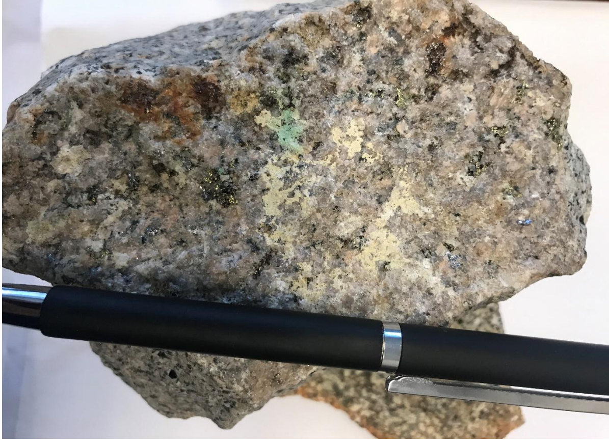
Figure 7, granodiorite with chalcopyrite and malachite alteration from Primary Ridge
