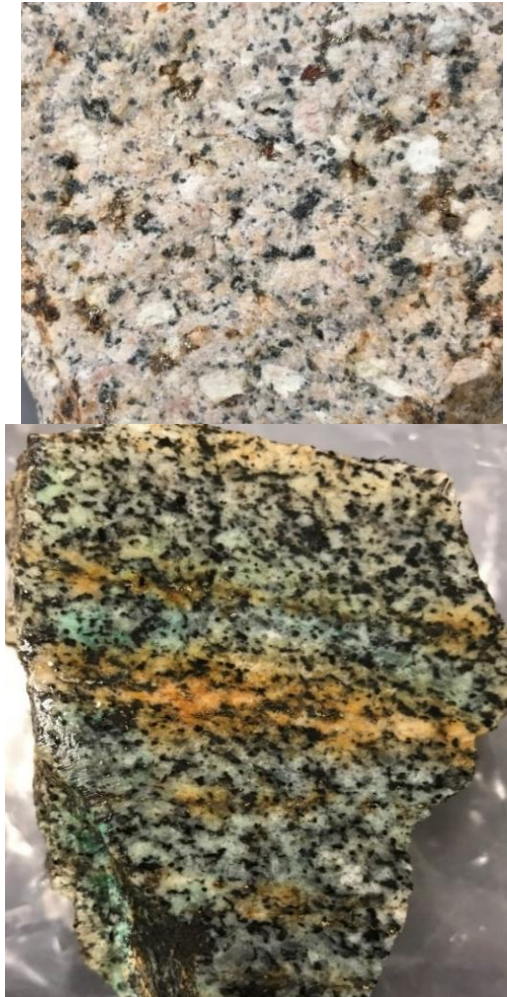
Figure 4, left, sample 719511 from Razorback porphyry area, tonalite with chalcopyrite and malachite alterations, showing B-veinlet crossing cut biotite and magnetite veins; right, sample A0020311 from Primary Ridge, monzonite with pyrite, showing strong potassic alteration
