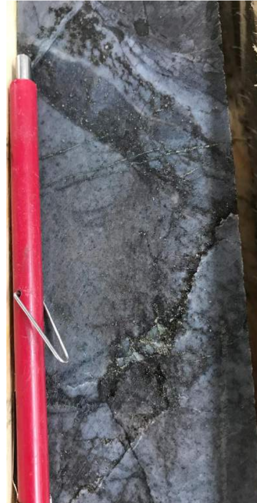
Quartz tourmaline breccia with pyrite at grade of 2.43 g/t Au, 0.06% Cu, 0.025% Co and 0.018% Bi
