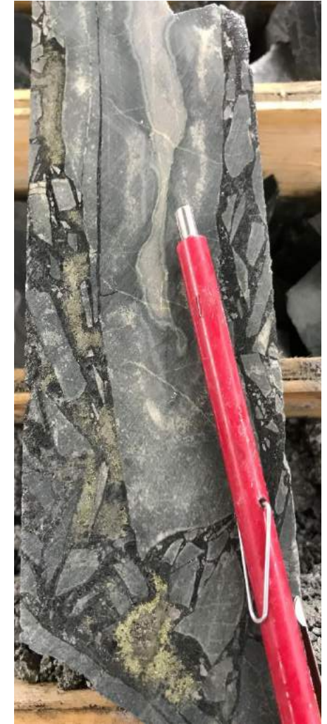
Tourmaline breccia with chalcopyrite at grade of 1.94 g/t Au, 0.13% Cu and 0.014% Co
