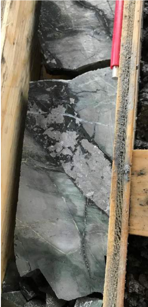
Tourmaline breccia with arsenopyrite at grade of 6.60 g/t Au and 0.10% Co
