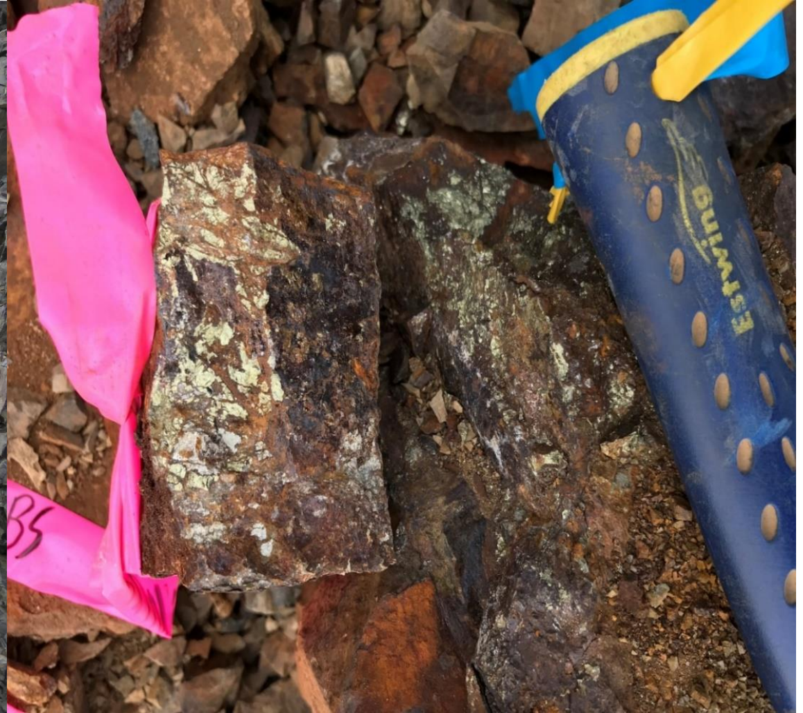
Massive sulphide (chalcopyrite) mineralization in tourmaline breccia zone (above)
