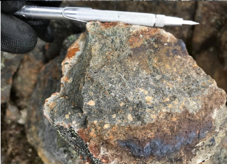
Pyrite veins, quartz veins stockworks in Hornfels and Pyrite/limonite in Granite
