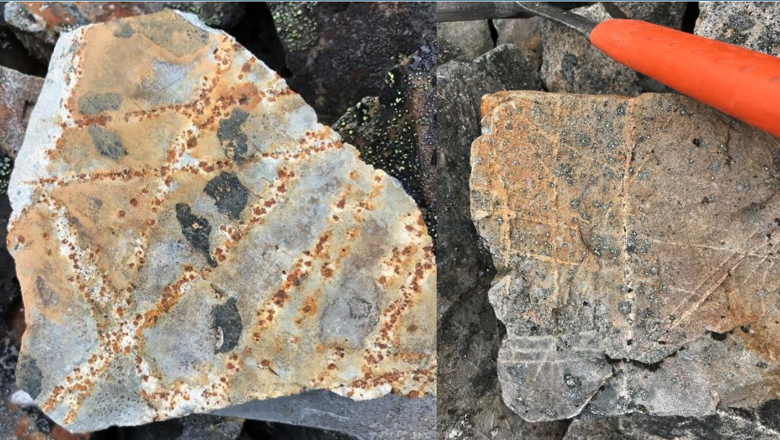
Pyrite veins, quartz veins stockworks in Hornfels and Pyrite/limonite in Granite
