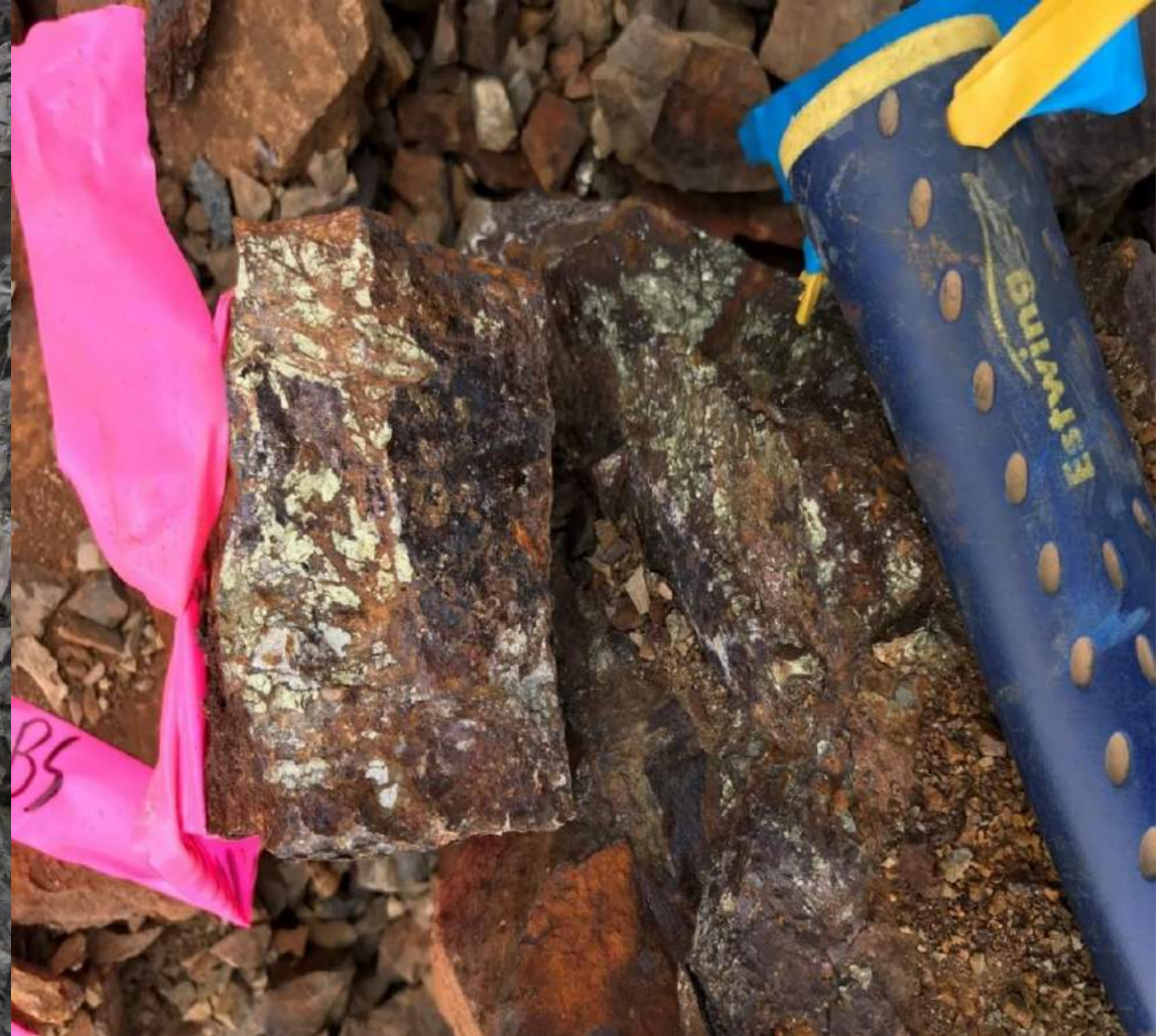
Massive sulphide (chalcopyrite/arsenopyrite) mineralization in tourmaline breccia zone
