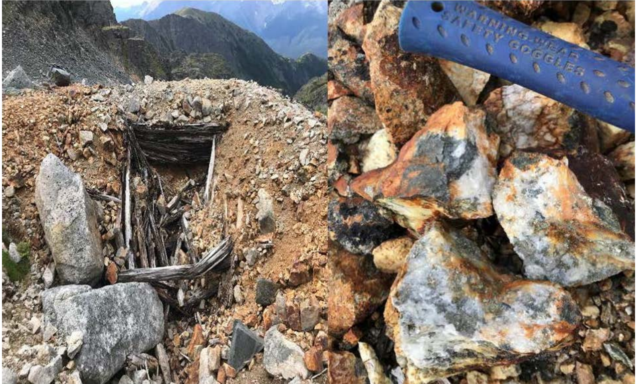
Figure 5. Artisanal Adit 1 (Left); Massive Sulfide Quartz Vein Ores (Right)
