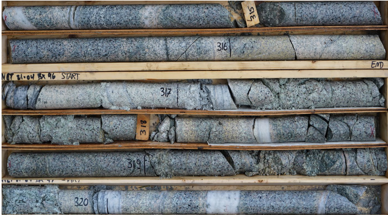
Figure 6. Core from 314.4 m to 320.8 m at NET21-04 showing the multiple sulfide quartz vein zone and intense potassic alteration in the granodiorite.
