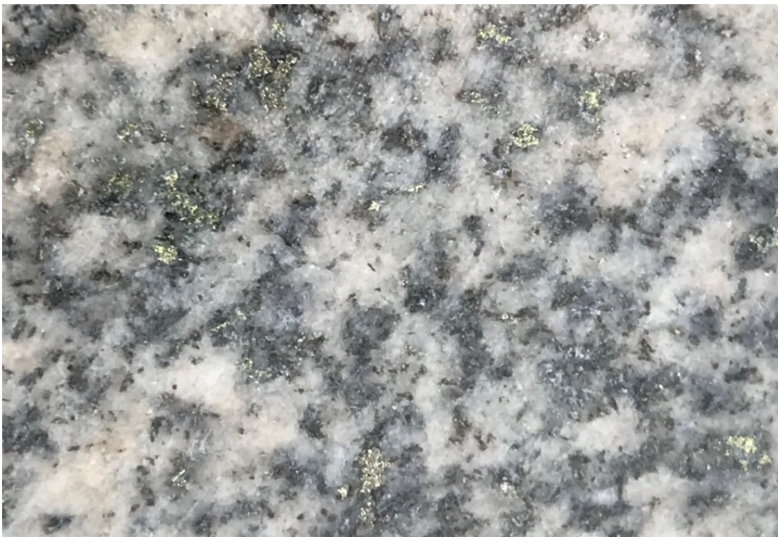
Figure 3. Cut core at 165.1 m at NET21-04 showing disseminated chalcopyrite and pyrite within monzonite porphyry.
