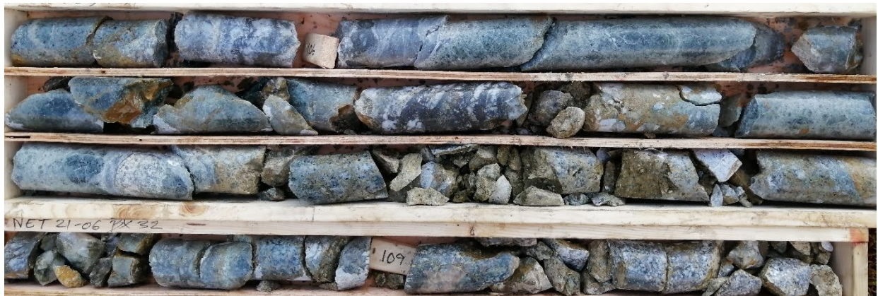
Figure 9. Core from 105.7 m to 109.5 m at NET21-06 showing the strong altered sulfide quartz breccia veining zone in the granodiorite.
