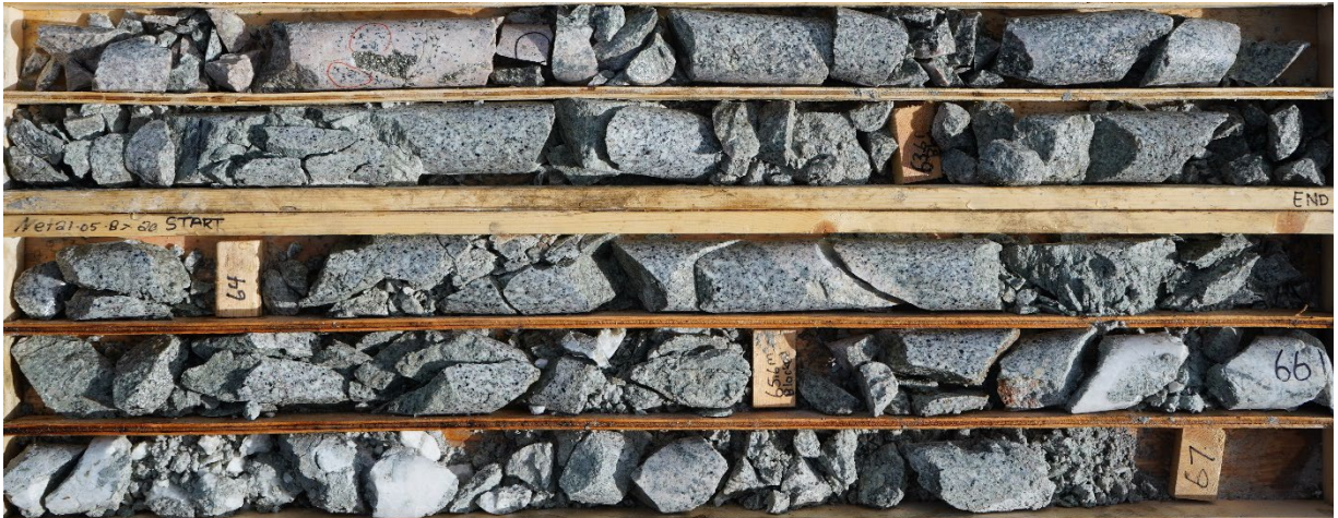
Figure 8. Core from 62.0 m to 67.0 m at NET21-05 showing the multiple sulfide quartz vein zone and intense potassic alteration in the granodiorite.
