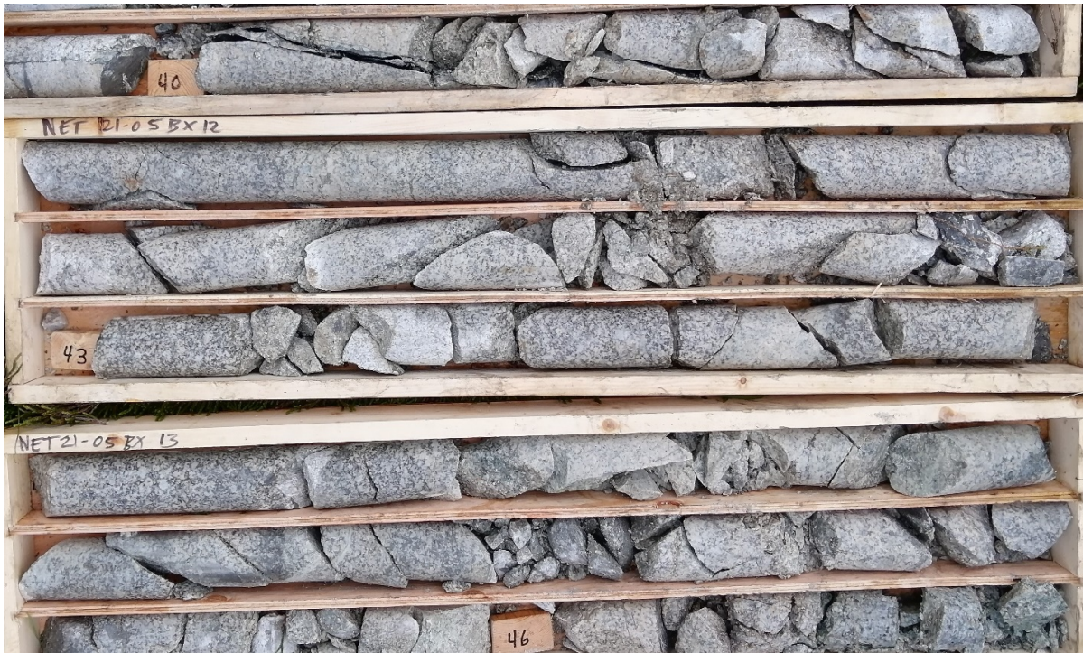
Figure 4. Core from 40 m to 46.6 m at NET21-05 showing sulfides monzonite porphyry dyke.
