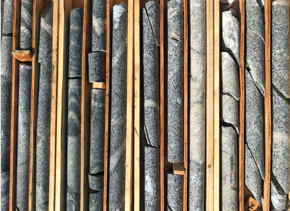
Figure 2. Core from 164 m to 176 m at NET21-04 showing multiple sulfides monzonite porphyry dykes and potassic alteration.
