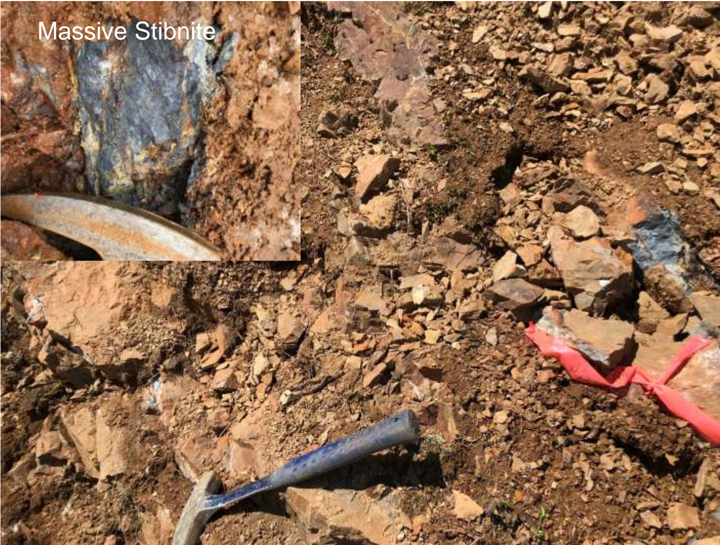
2 m thick massive Sb sulfide vein @ 6.48% Sb
