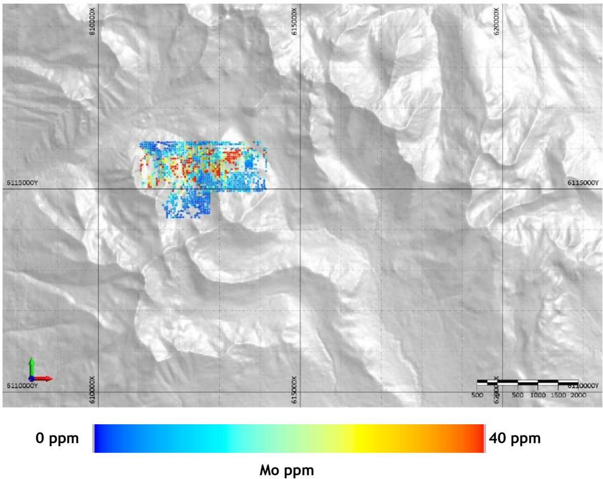
**Figure 1:** Soil sample locations for the Red Springs project area colored by Mo concentration. The Mo values are quite high in the area. The rocks samples for the area cover a larger region as indicated in **Figure 2**.
