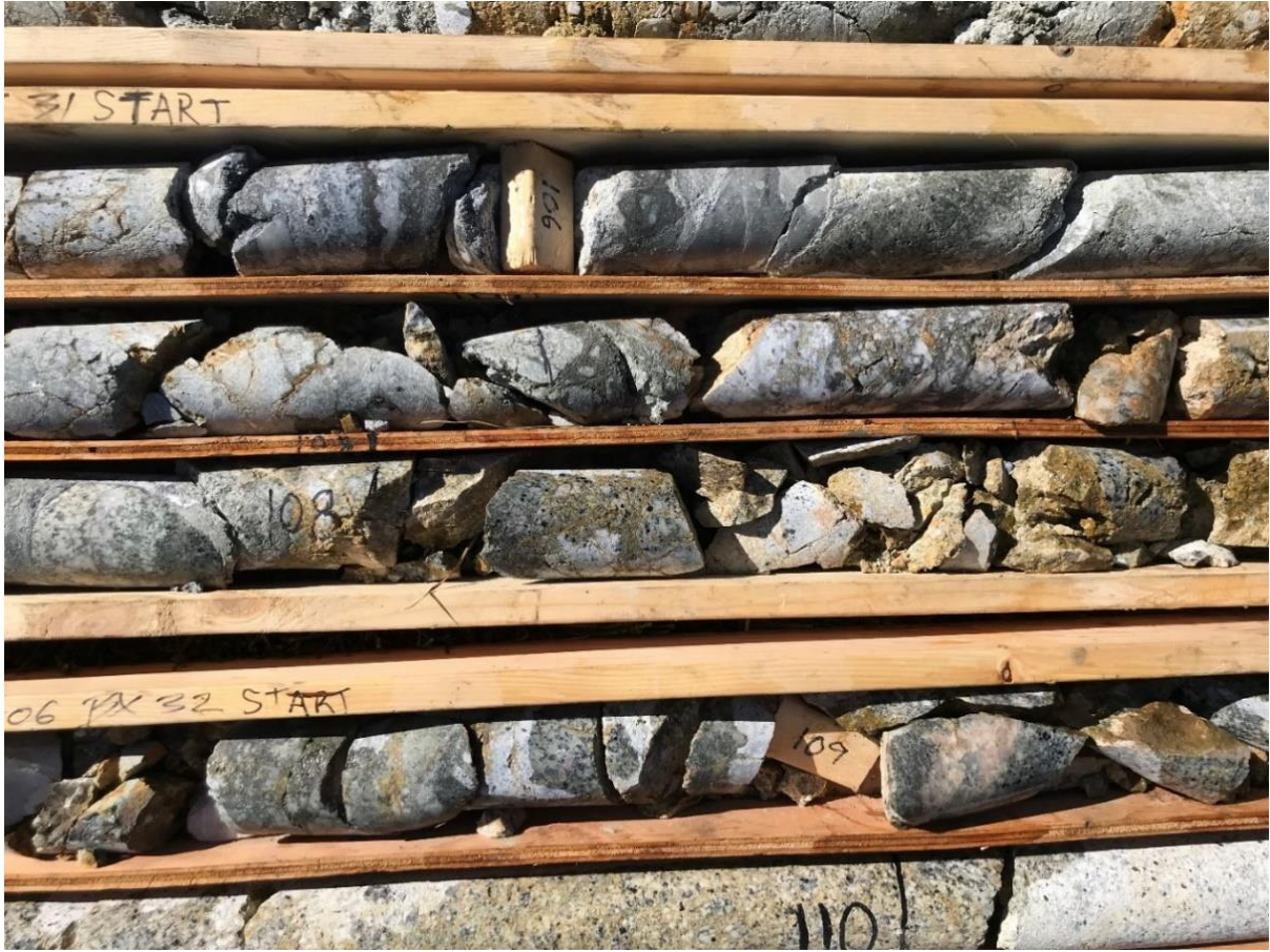
Figure 3. Core from 105.7 m to 109.2 m at NET21-06, showing strong disseminated chalcopyrite and pyrite within monzonite porphyry dyke, quartz veins breccia and sulfide quartz veins. Three spot counts at 107.0-107.20 m returned over 752 g/t Ag, 1.8% Cu, 1.2% Zn and 0.46% Sb.
