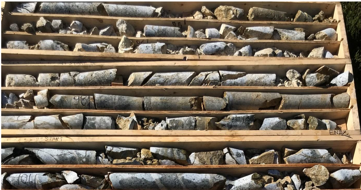
Figure 4. Core from 93.5 m to 100.5 m at NET21-06, showing multiple sulfide quartz vein zones and monzonite dykes; one large dyke from 98.0 m to 99.2 m showing strong disseminated and vein sulfides and silicification.
